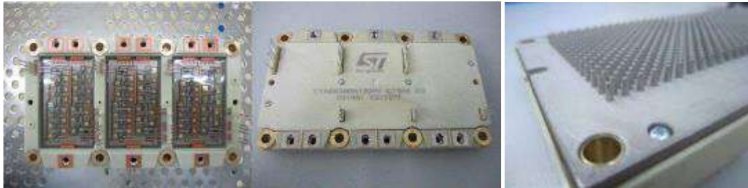
Figure 32 Inverter module prototype – target is to reduce the global weight of 25-30%
