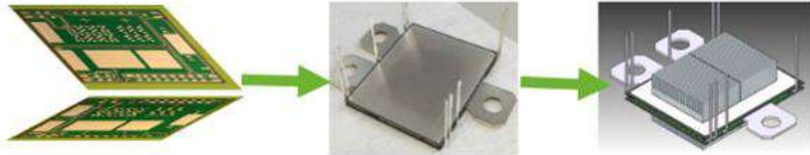
Figure 28: A new generation of Power Module (here 3D)
