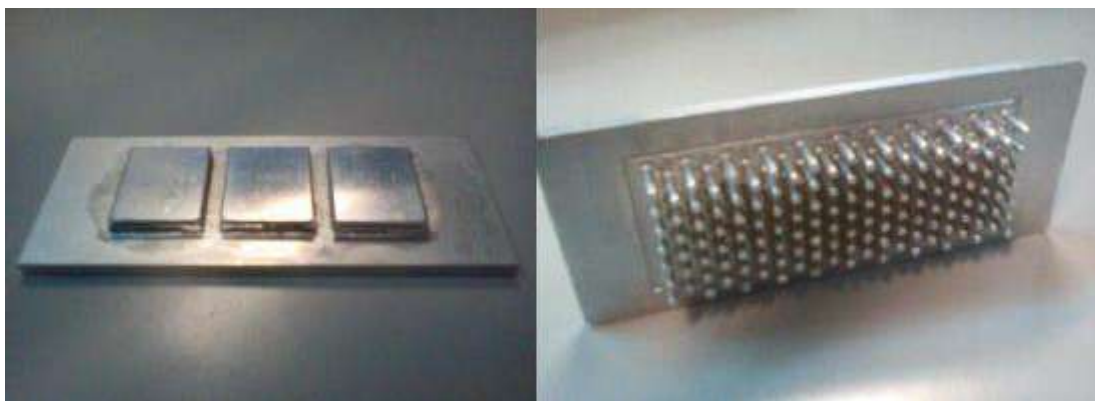
Figure 33 Grinding to move from current state of art of 110 µm thickness up to 50 µ reducing Rth
