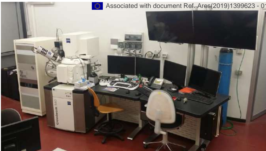
Left: Lenton UAF 17/12M vertical Furnace used for the calcination process. Right: Zeiss Crossbeam 540, Dual Beam SEM/FIB electron microscope
