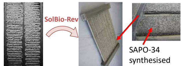
Fig. 17. Left: standard loose-grains adsorber. Right: envisaged coated adsorber HEX
