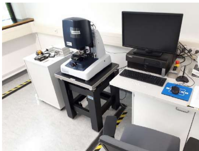
White light interferometer (WLI) and profilometer for surface characterisation of printed TEGs at KIT
