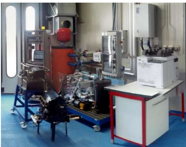
Left: Small-scale adsorption chiller prototype testing. Right: Adsorber HEX characterisation testing-rig
