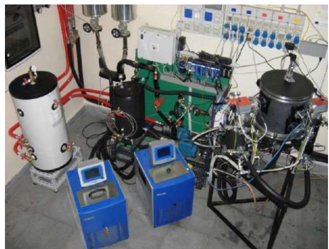
Left: Small-scale adsorption chiller prototype testing. Right: Adsorber HEX characterisation testing-rig
