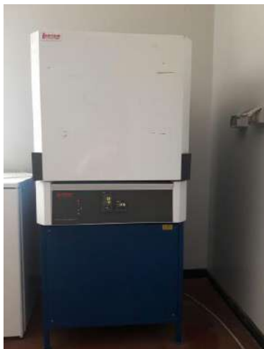
Left: Lenton UAF 17/12M vertical Furnace used for the calcination process. Right: Zeiss Crossbeam 540, Dual Beam SEM/FIB electron microscope
