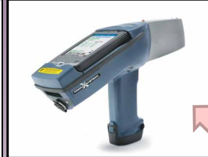
Handheld XRF 'Alpha 4000' (Innov-X System) analyzer
